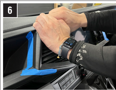
6 Remove the trim around the top, bottom and vents to release the panel. See step 7, which highlights the clips that secure the trim panel.
