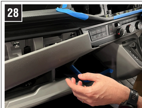
Remove the panel above the glovebox using a panel removal tool to release the clips highlighted in step 29.
