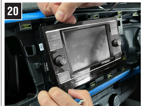
20 First, release the left-hand side of the head unit; once released, use the release keys to remove the opposite side.
