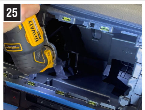
Ensure the area that is being cut is clear of any wires.
