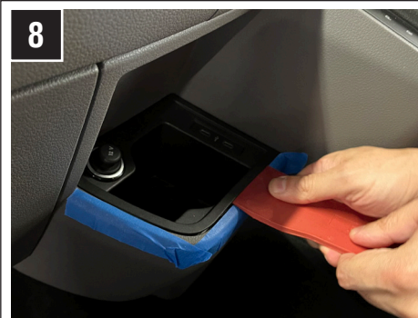
8 Use a panel removal tool to remove the panel which houses the OEM USB ports, this is secured with clips in each corner. (see step 9)
