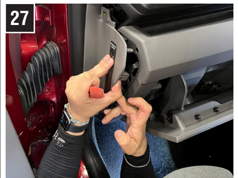
To remove the glovebox, first remove the side panel with a panel removal tool.
